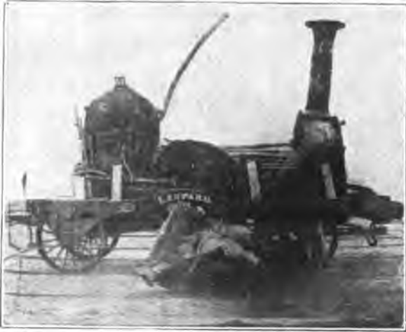
Fig. 106.—"Leopard," from a photograph taken after an explosion in 1857.
